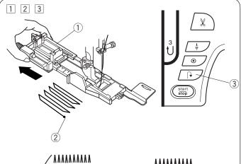
1 Attach the automatic buttonhole foot R and pull the button holder all the way out.
