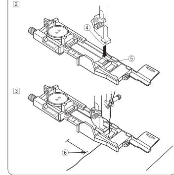
The size of a buttonhole is automatically set by placing a button in the rear of automatic buttonhole foot R.
