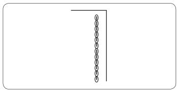
This strong, durable stitch is recommended for areas where both elasticity and strength are needed to ensure comfort and durability. Use it to reinforce areas such as crotch and armhole seams. Also use it when constructing items such as backpacks for extra strength.
