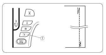
Use this stitch to secure the beginning and the end of a seam with backstitching. When you reach the end of the seam, press the reverse button ① once. The machine will sew four reverse stitches, four forward stitches, and then stop sewing automatically.
