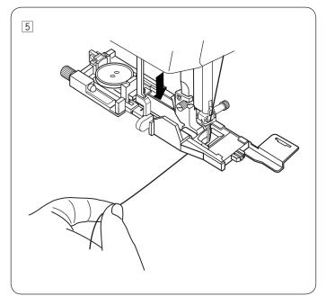
5 Start sewing while pulling the needle thread lightly to the left. After sewing a few stitches, free the thread and continue sewing.
