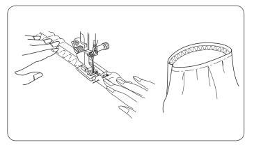
Mark the elastic into quarters. Match those to the center front, center back and side seams, and pin the elastic to the fabric.
