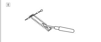
8 Place a pin just below the bartack at each end to prevent accidentally cutting the threads. Cut the opening with the seam ripper. Use an eyelet puncher to open a keyhole buttonhole.
