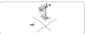
You can close quilt layers by using the clasp stitch. Select stitch pattern 06 (mode 2). Press the memory key. Select locking stitch (pattern 87 (mode 2)).
