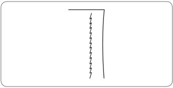
This is a narrow stretch stitch in the left needle position designed to eliminate puckering on knit fabrics and bias seams, while permitting the seam to be pressed completely open flat.
