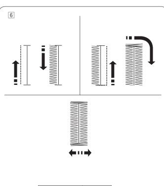
6 The buttonhole is sewn automatically in the sequence shown. When the buttonhole is finished, the machine will stop automatically with the needle in the up position.
