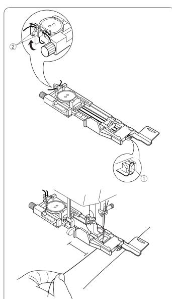
Place the button on the button holder on the buttonhole foot.
