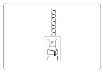
Sew a fine seam in lingerie and lightweight knits. The small seam size stretches and is comfortable to wear.
